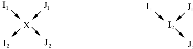
Figure 5 There are no choke points between \{I_1, I_2\} and \{J_1, J_2\} in either of these graphs, though there is a weak choke point in both cases: X on the left and I_2 on the right. On the left, X is not on the \{I_1, I_2\} side of \langle I_1 X J_2 \rangle , and not on the \{J_1, J_2\} side of \langle I_2 X J_1 \rangle . On the right, I_2 is not on the \{I_1, I_2\} side of \langle I_1 I_2 J_2 \rangle , and not on the \{J_1, J_2\} side of \langle I_2 J_1 \rangle .
